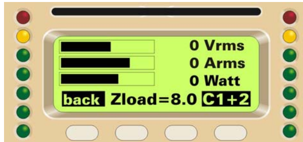
C1+C2 shows the output values are being shown in bridge mode.
